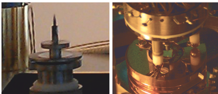
Figure 2.3: Photograph on the left panel shows a single piezo tube scanner from the Omicron LT-STM. The tip is pointing upwards. The right photograph shows a Variable Temp Beetle TM type scanner placed over a sample holder from the RHK STM. Here, the tip is pointing downwards.
